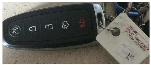
Submission the FCC ID from one of the example key fobs to <a href="http://fccid.io">http://fccid.io</a> results in details for the fob including the transmission frequency, internal photos, and circuit schematics.
