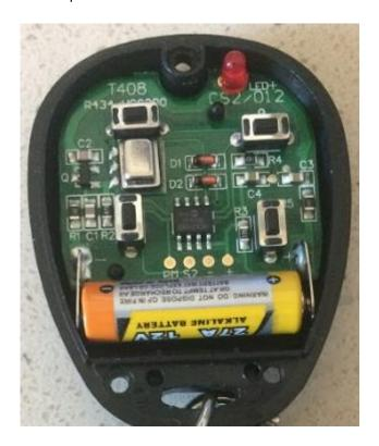
Inspecting the components on the internal circuit board, the central component that operates the device is a MicroChip HCS200 integrated circuit. A Google search on this device reveals the datasheet that engineers use to integrate the component into their designs.
