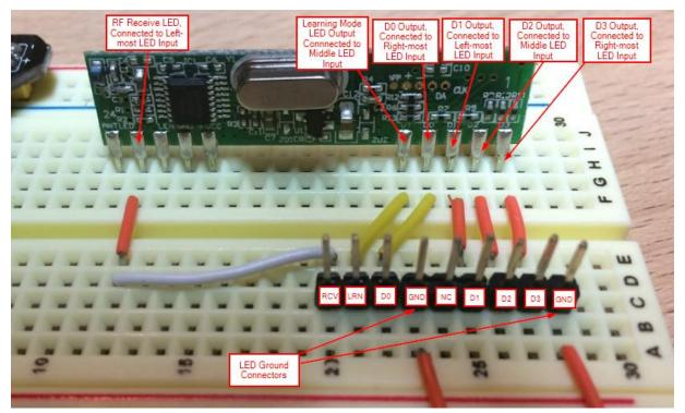
Finally, connect the Pi-Stop LEDs to the exposed headers with the Gnd pin to the right as you are facing the header with column C of the breadboard closest to you.
