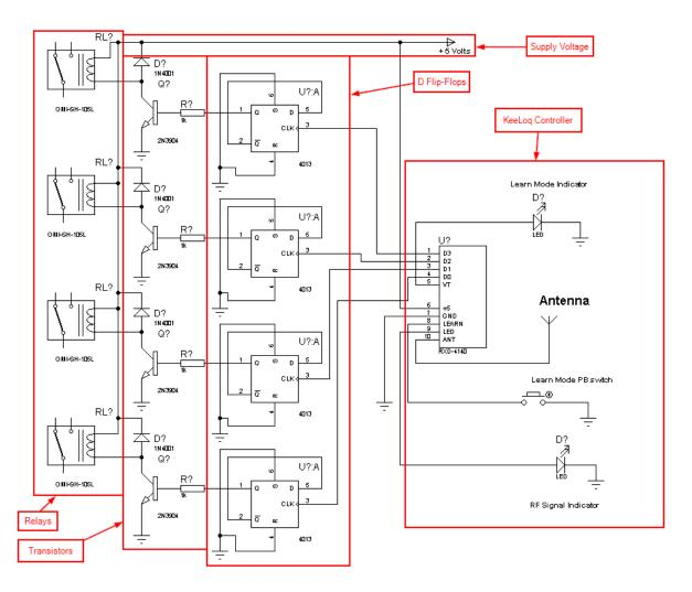
In this diagram, the device is wired up to four D flip-flops, one for each output, that simply serve to remember the state of the output. The outputs of the flip-flops are then connected to transistors that supply current to a relay. The relay is used to connect the 5V device to the 12V circuitry of the vehicle and activate the intended feature.
