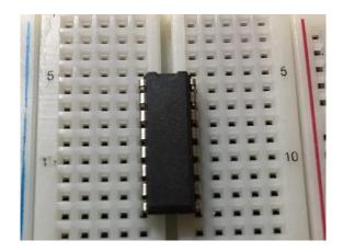
With a basic understanding of breadboard organization, you can begin wiring up the KeeLoq circuit. Insert the KeeLoq controller into the pins column H on the mini breadboard. This isolates the pins from one another and allows us to connect other components to the inputs and outputs of the device.
