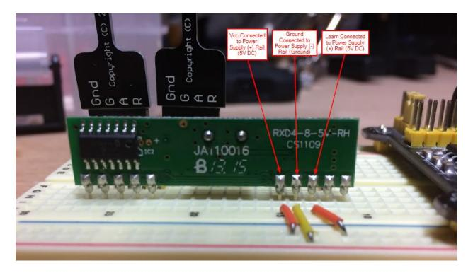
On the reverse side of the KeeLoq device, connect the three inner pins as identified above. These are Vcc, Ground and Learn. Vcc provides power to the device and should be connected to the power supply + rail. Ground allows current to exit the circuit and should be connected to the power supply - rail. The learn input is not used for our purposes. However, this input is "active low" meaning that it must be held at 5V to avoid being placed into learning mode.
