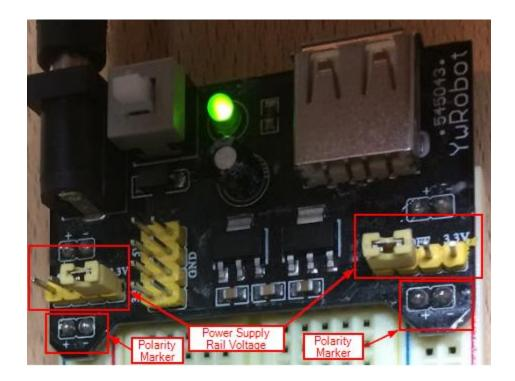
The jumpers in the image above should be set to 5V. This controls the voltage placed on the supply rails. Notice polarity markers on the power supply rails. As you are constructing the circuit you must be careful to connect the Vcc and Ground connections properly. On this particular breadboard, the blue side of the rail is Vcc (5V) while the red side of the rail is Ground.
