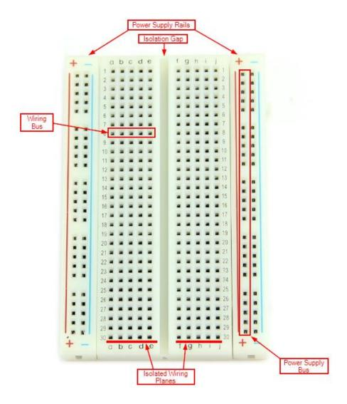
The isolation gap is used to accommodate Dual In-line Package integrated circuit components like the one seen below. This allows a circuit designer to easily isolate the pins on the chip and provide discrete inputs to each.
