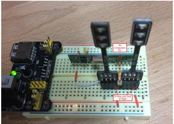
After checking each of the connections, you should be able to power on the breadboard and use the key FOB to activate each of the LEDs on the Pi-Stop.
